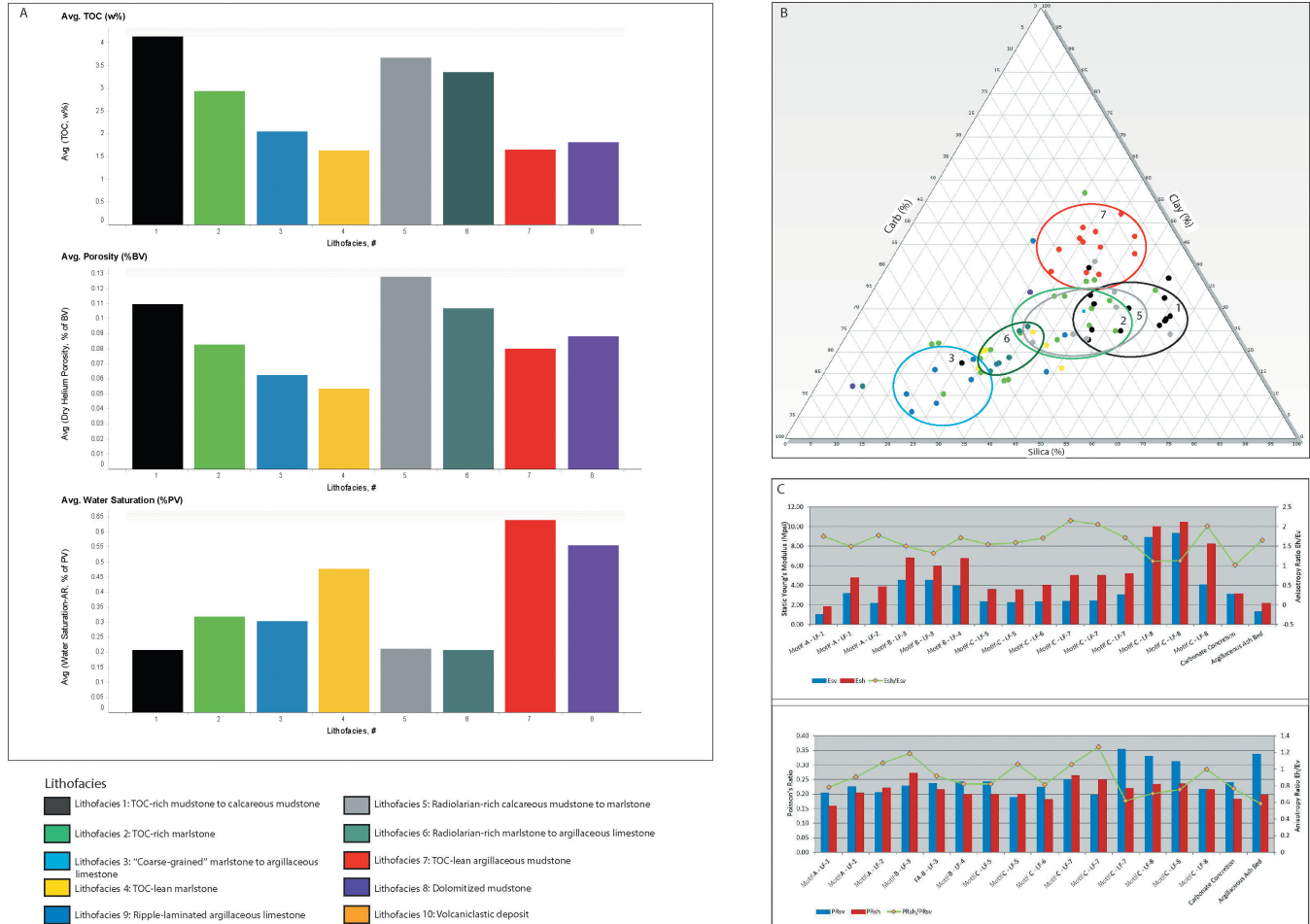
Figure 13. (A) Lithofacies plotted against TOC, porosity, and water saturation. (B) XRD analyses of core samples plotted in a ternary diagram silica–carbonate–clay and grouped by lithofacies (compare colors and numbers with [A]). (C) Lithofacies plotted against Poisson’s ratio (above) and static Young’s modulus (below); both plots show Anisotropy Ratio (green line), PR_{SV} (blue histograms), and PR_{SH} (red histograms).
